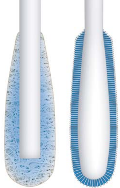
Traditional fiber swab comprising fiber wad
